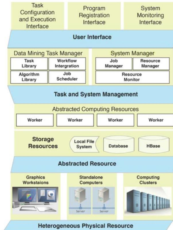
Figure 1: FIU-Miner System Architecture
