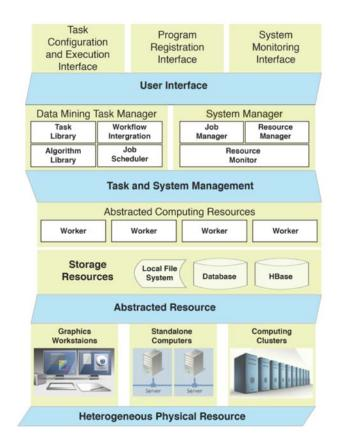
Figure 1: FIU-Miner System Architecture
