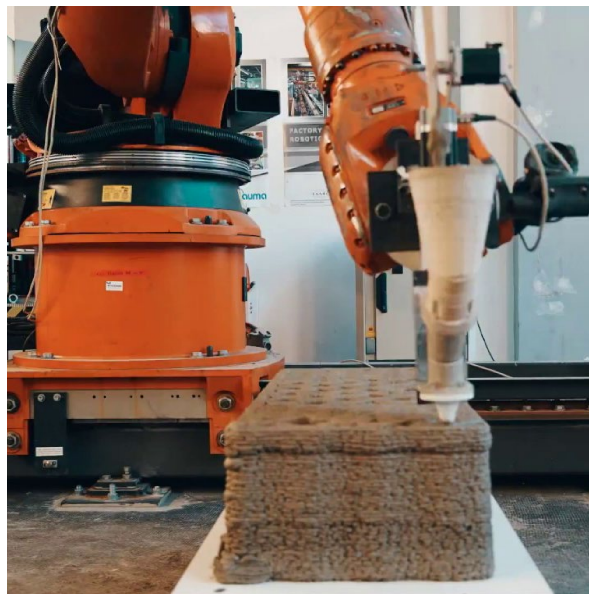
Figure 1. Example of an existing concrete extruder attached to a robotic arm
