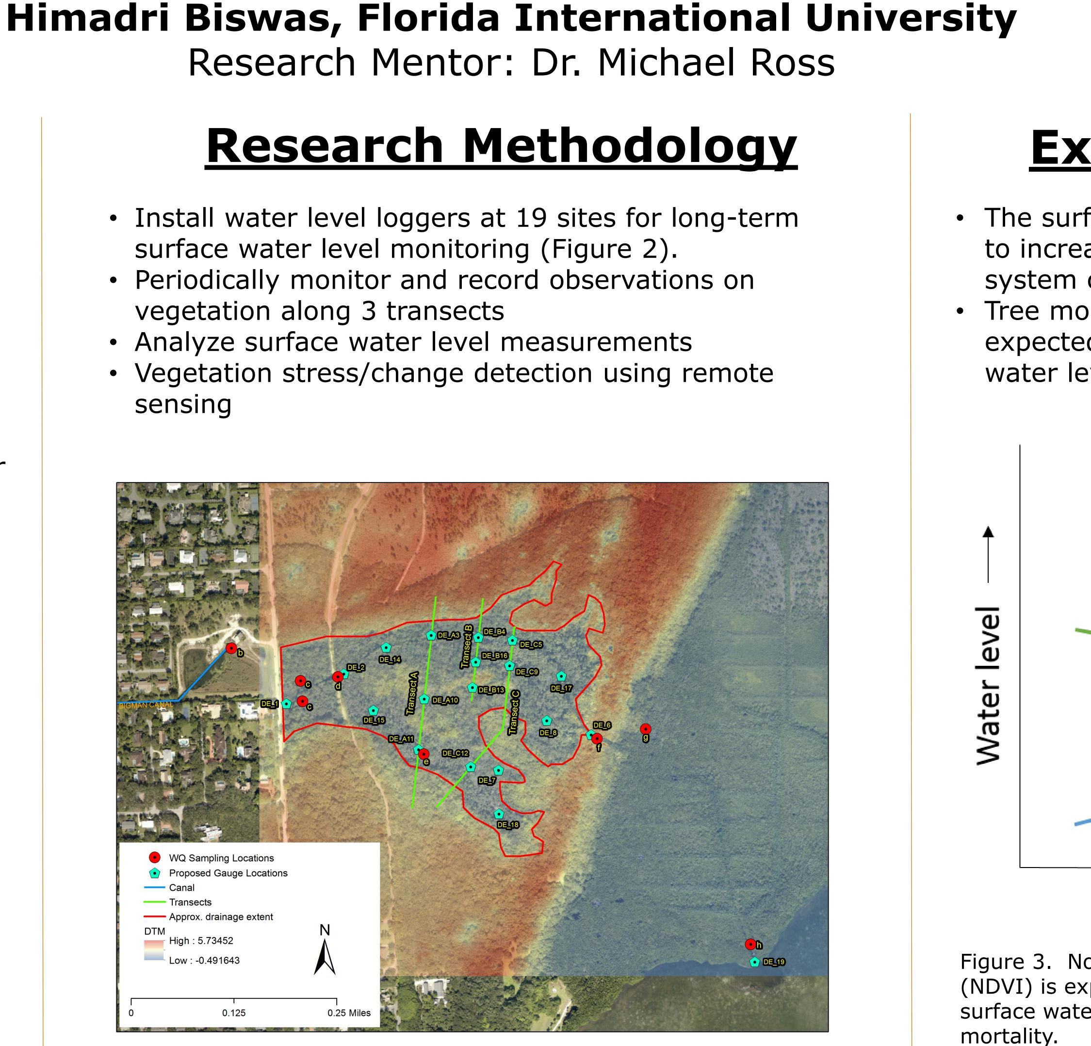
Figure 2. Proposed gauge locations to monitor the surface water level
