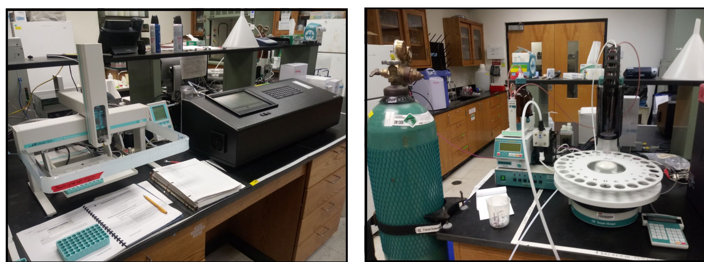
Figure 2. Auto-injector and Liquid Water Isotope Analyzer (left), Titrator (right).
