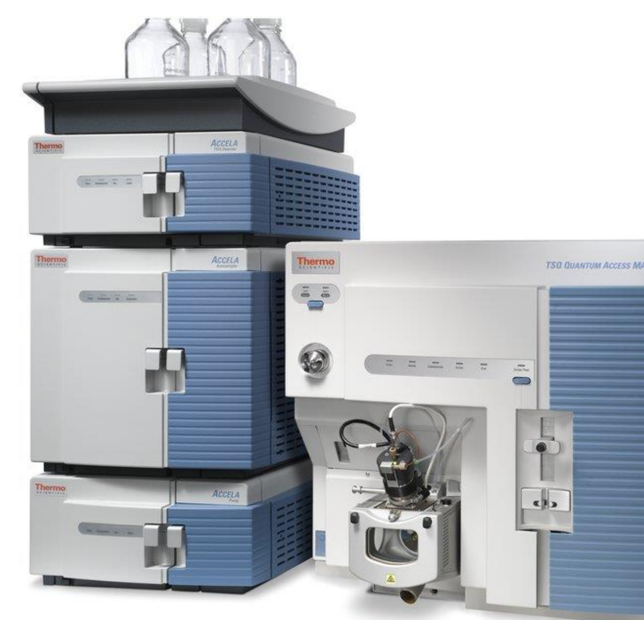
Figure 4. LC-TSQ. Parameters – Ionization: ESI; Polarity : Negative; Spray Voltage: 5 KV; and Capillarity temperature: 350°C
