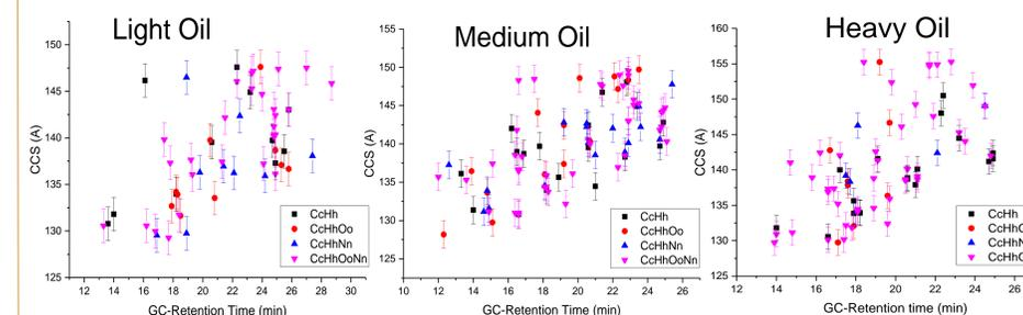
Figure 7: Typical plot of CCS vs. GC retention time of the PAH SARA fraction of three common crude oils (m/z range 160 – 215). The bar represents the FWHM of the GC and CCS peaks. Notice the isomeric complexity
