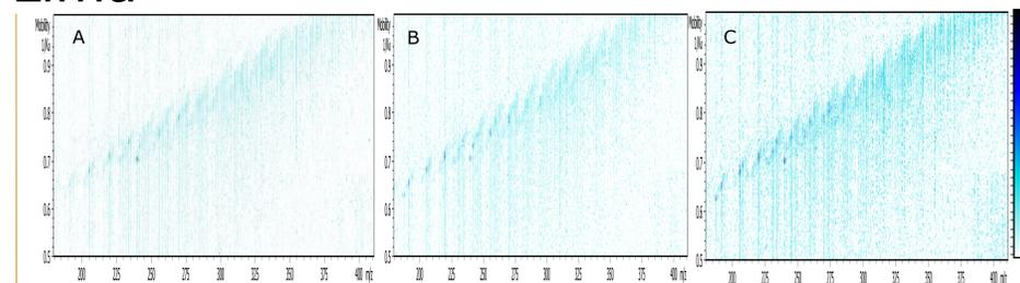
Figure 4: Typical 2D-IMS-MS contour plot of the PAH SARA fractions of three common crude oil samples analyzed by GC-APLI-TIMS-MS: (A) light oil (B) medium oil (C) heavy oils
