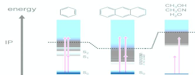
Figure 1. Scheme of the multi-photon ionization process utilized for the analysis of polyaromatic hydrocarbons (PAHs) during GC-APLI-TIMS-MS.
