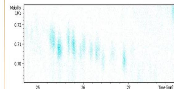
Figure 5: Typical 2D-IMS-MS contour plot at 220 m/z from the PAH SARA fraction of a light oil. Notice the complexity at the level of nominal mass and the orthogonality between GC and TIMS in the separations.
