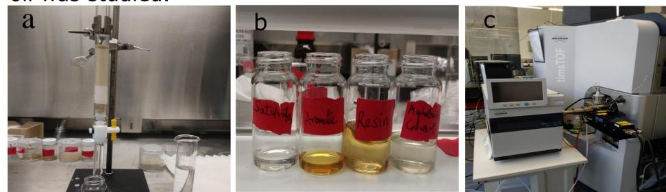
Figure 2. Typical SARA column (a) and fractionation products (b). Illustration of the GC-APLI-timsTOF instrument utilized in this study
