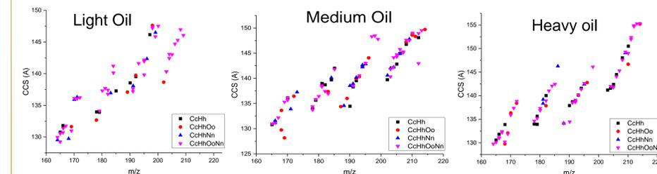
Figure 6: Typical plot of CCS vs. m/z of the PAH SARA fraction of three common crude oils. The plot shows the prevalence of  $C_cH_hO_oN_n$  class in the 160 – 215 m/z range.
