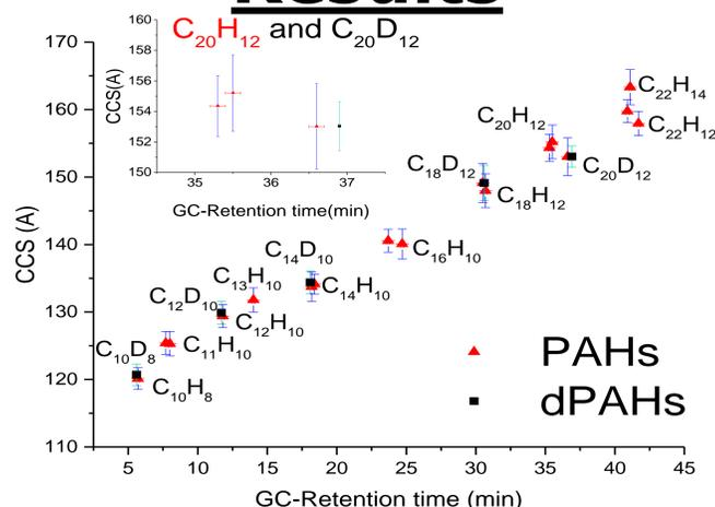
Figure 3: Typical plot of CCS vs. GC retention time of PAH and dPAH standards. The bar represents the FWHM of the GC and CCS peaks. Notice the complementary separations between GC and TIMS for  $C_{20}H_{12}$  and  $C_{20}D_{12}$  isomers (inset)
