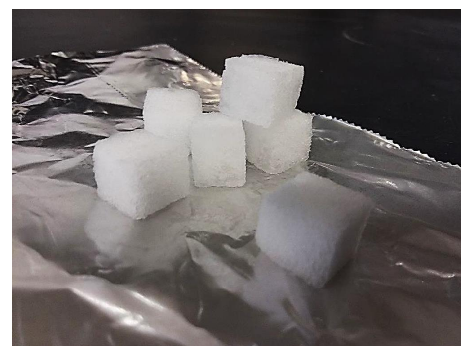
Figure 2. Resulting PDMS sponges from the above illustrated process.
