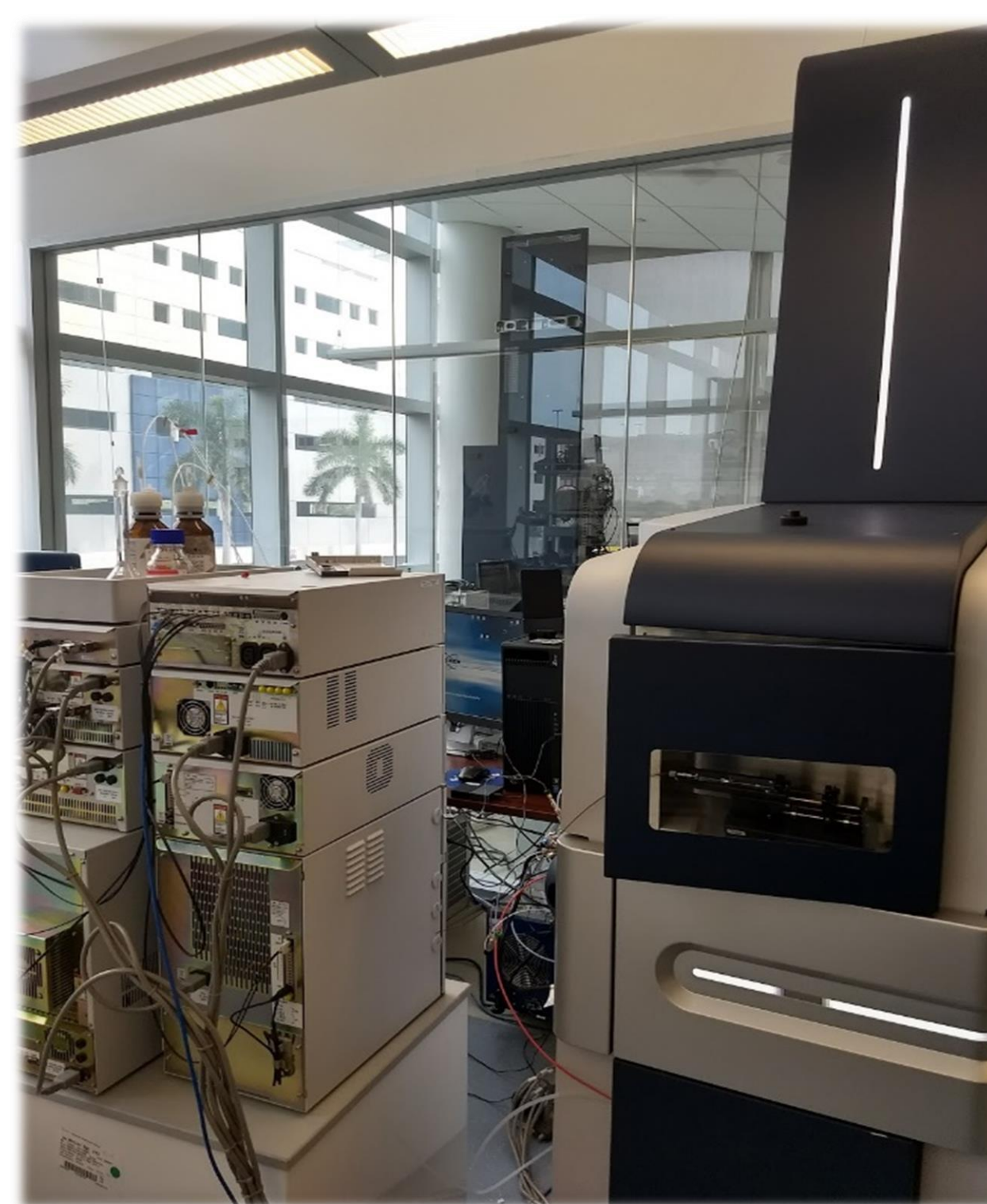
Figure 2. Bruker LC-MS/MS instrument
