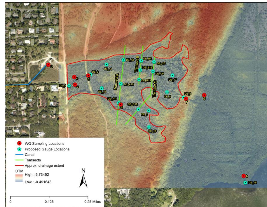
Figure 2. Proposed gauge locations to monitor the surface water level
