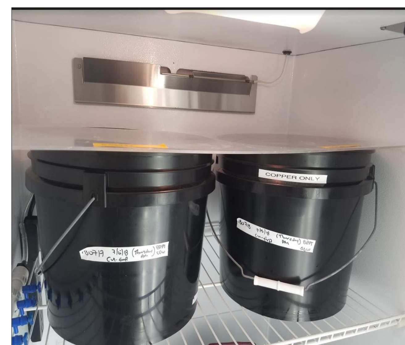
Figure 6. Acute copper experiments. Fish were exposed to 11.1 or 0 (control) µg/L copper for 96 h with renewals at 48 h. During exposure, fish (N= 11 per treatment) were kept individually in buckets at 25 °C in an incubator.
